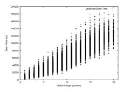
**Fig. 1.** The Impact of Queue Length on Drain Time: Scatter plot of observed values. Testbed setup as in Section 2, scenario described in Section 3.
