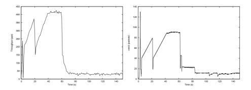
Fig. 10. TCP Vegas with an additional 200ms RTT in an initially uncontended network with additional fbws introduced at 60s: (a) throughput, (b) cwnd.
