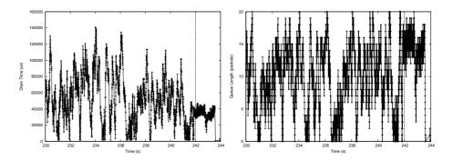
**Fig. 6.** The impact of other stations leaving the system: (a) drain times and (b) queue lengths. At time 242s other stations have stopped.
