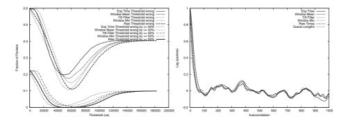
**Fig. 5.** Thresholding of filtered delay measurements: (a) errors while thresholding simple measurements, (b) autocorrelation of filtered measurements.
