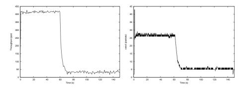
**Fig. 9.** TCP Vegas wth 5ms additional RTT in an initially uncontended network with additional fbws introduced at 60s: (a) throughput, (b) cwnd.
