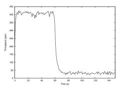
Fig. 8. Throughput for TCP Reno in an initially uncontended network with additional fbws introduced at 60s.
