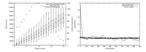
**Fig. 3.** Statistics for drain time against queue size (a) 10–90% box-and-whiskers plot and mean. The number of samples is also shown on the right hand axis, (b) autocorrelation for the sequence of MAC service times, queue drain times and queue lengths.
